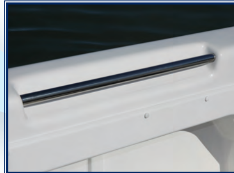
Sturdy stainless steel grab rails are recessed into the gunwales for maximum strength
